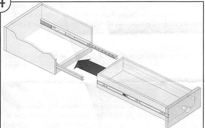
4. Insert drawer into cabinet and close. The drawer slide release lever will lock as drawer is closed. Make sure drawer aligns properly and rides smoothly on the side mount drawer slides.
