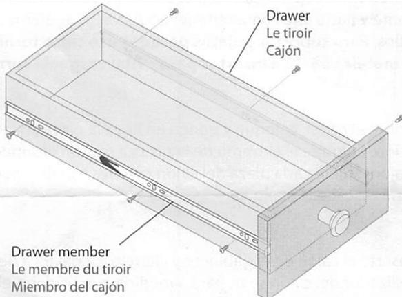
3. On drawer place and align drawer member into position. Place drawer member end flush with the drawer overlay. Fasten each drawer member with (3) #6 pan head wood screws.
