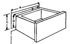
Make drawer dimension "B" 1" to  $1 \frac{1}{16}$ " narrower than opening dimension "A", and depth dimension "D"  $\frac{1}{4}$ " minimum less than opening dimension "C".
