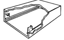
Mount cab members CL & CR flush with front and bottom of casing.
